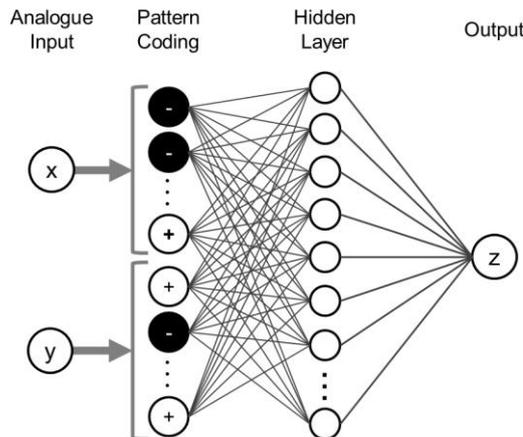
Fig. 4. Structure of pattern coding-applied MLP (MLP-P).
