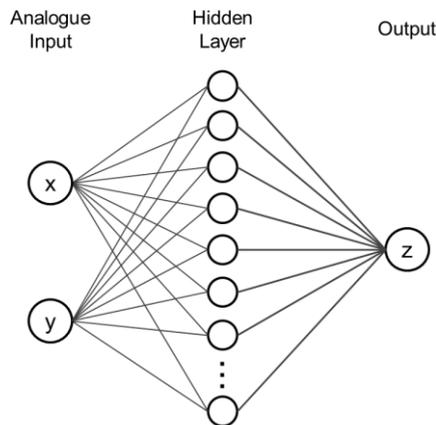
Fig. 3. Structure of an ordinary MLP that uses analogue input (MLP-A).
